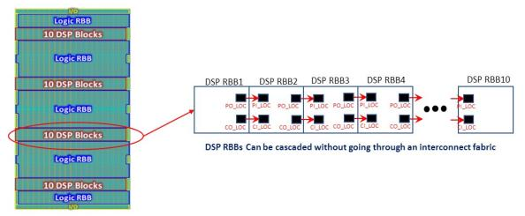
The 40 DSPs in an EFLX4K are in rows of 10 DSP RBBs.  $P_{out}$  of one DSP pipes to  $P_{in}$  of the adjacent DSP. This improves performance for many DSP functions.
