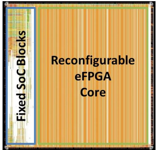
Fig. 5. Chip layout of the DragonFly rad-hard System-on-Chip, showing fixed IP blocks and a reconfigurable embedded FPGA core.
