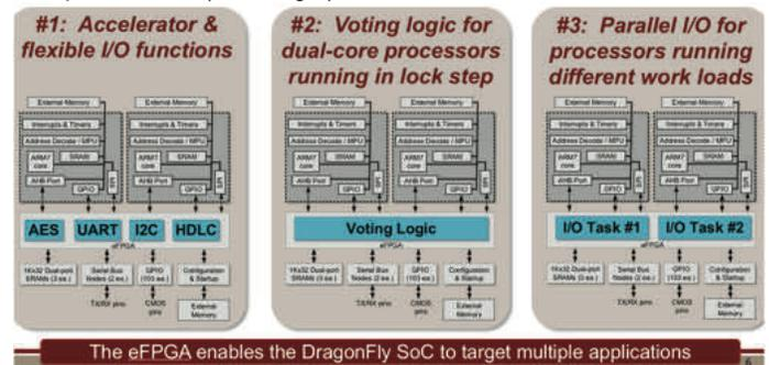
The eFPGA enables the DragonFly SoC to target multiple applications
