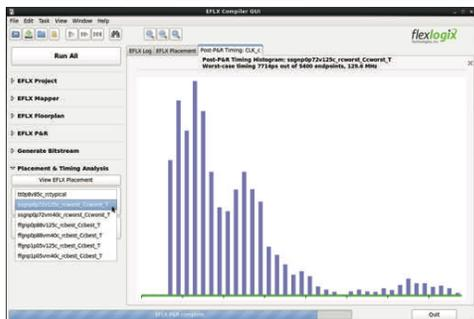
Above and to the left are some screen shots from the EFLX Compiler GUI. Above left shows the screen for selecting the array size in number of rows and columns; and which tile are Logic, DSP or IO. In the middle is a 5x5 array that has been placed. Above right is a timing browser for examining/debugging critical paths. And to the left is a timing histogram of all the critical paths in an array. These are just some of the GUI tools available for the designer.
