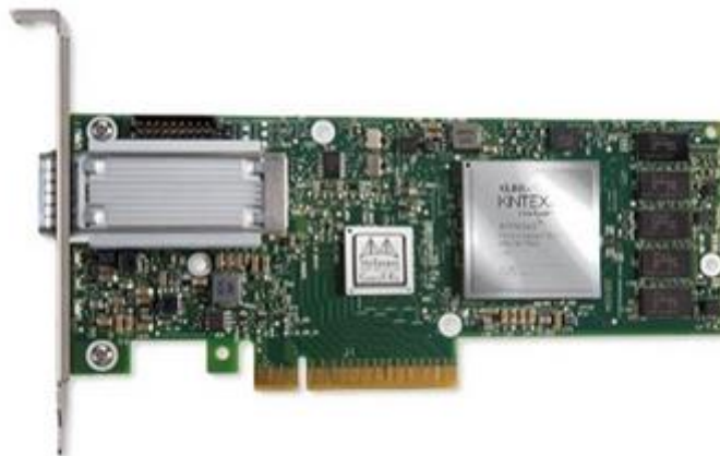
SmartNIC with network processor and FPGA
