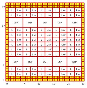
The EFLX 1K tile has 368 input pins and 368 output pins. The I/O pins provide user access to the EFLX tile. Each I/O has a bypassable flip flop. When multiple tiles are concatenated into EFLX arrays, the user I/Os along the abutting edges are disabled (or are used for controlling embedded RAM blocks).
