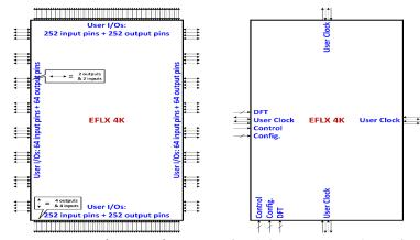
EFLX 4K Logic/DSP input/output map (IO tile has more IO top+bottom)
